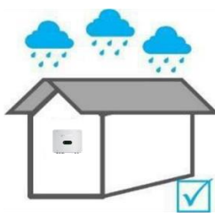
No rain exposure
